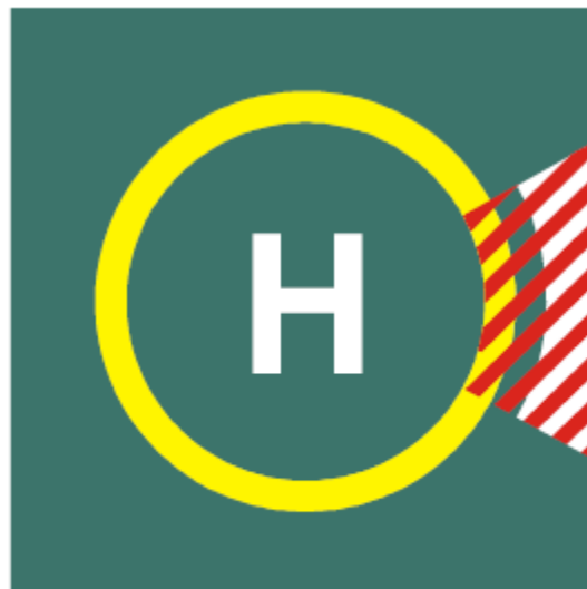
Figure 5-7. Helideck prohibited landing sector marking
